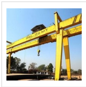
Goliath Gantry Crane
