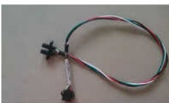
Lift Motor Position Sensor
