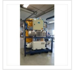
VPSA Nitrogen Generator
