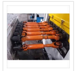
Steel Plant Cardan Shaft
